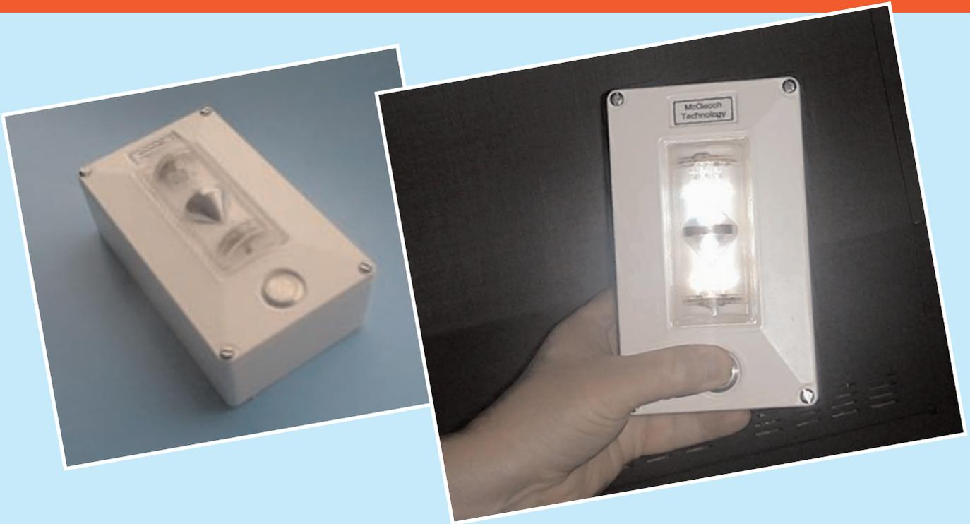
McGeoch Technology's **NEW** Automatic Emergency Lantern (AEL) is a solid state miniature unit utilising the very latest LED technology to provide controlled lighting over a 180° horizontal field of view. The unit is designed to illuminate for a minimum period of 6 hours following power failure. It will fully recharge within 16 hours of power being restored.
